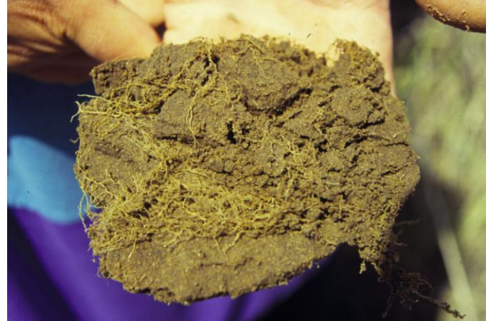
Note the compacted zone below the roots at the bottom of the photo. This compacted soil prevents roots from growing and can prevent water from infiltrating through the soil profile.
