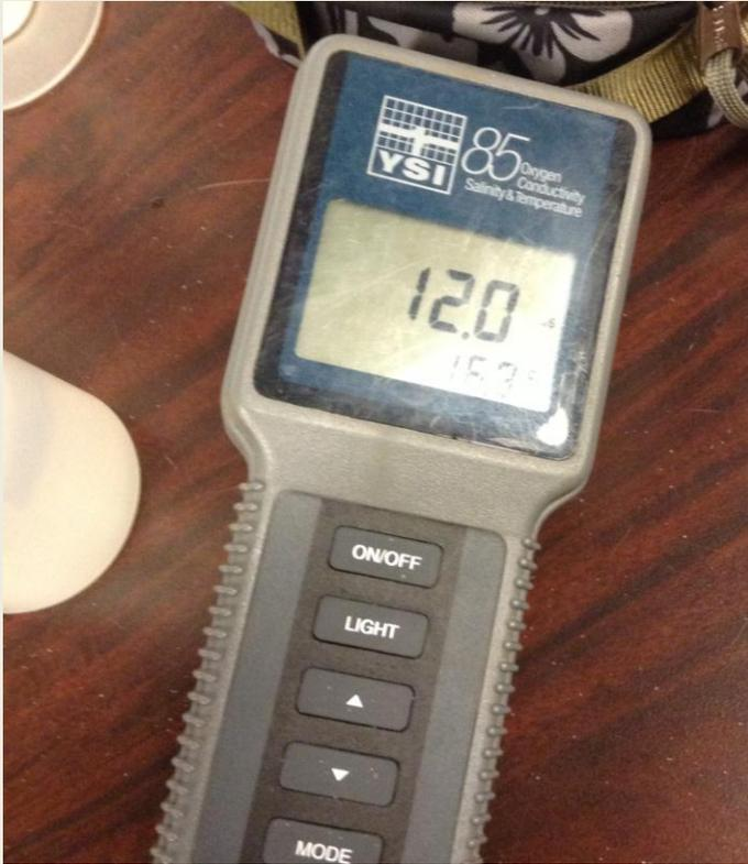
Using a conductivity meter, is an easy way to determine ion concentrations in sand (soil)
