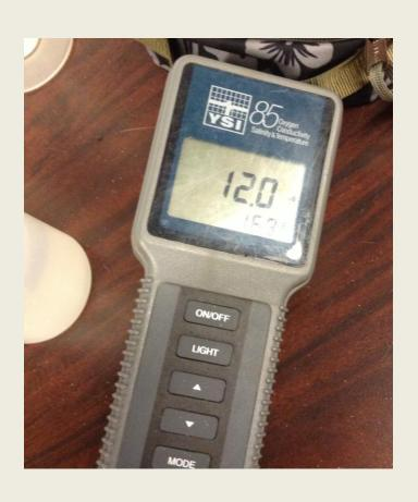
Using a conductivity meter, is an easy way to determine ion concentrations in sand (soil)
