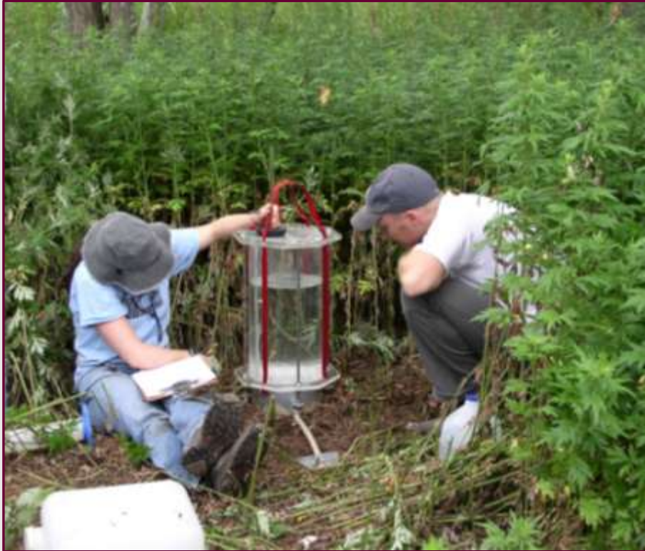
Cornell Sprinkle Infiltrometer Soundview Park - Low use area
